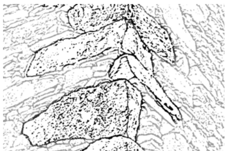
figure 24: placing of stones in a corner
